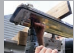
2. Attach a New Basic or Wide Reflector to the existing gear tray
